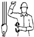
Travel (One Track) Lock the track on side indicated by raised fist. Travel opposite track in direction indicated by circular motion of other fist, rotated vertically in front of body. (For crawler cranes only.)
