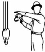
Move Slowly Use one hand to give any motion signal and place other hand motionless in front of hand giving the motion signal. (Hoist Slowly shown as example.)
