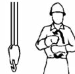
Travel (Both Tracks) Use both fists, in front of body, making a circular motion, about each other, indicating direction of travel, forward or backward. (For crawler cranes only.)
