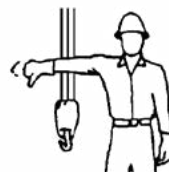
Lower the Boom and Raise the Load With arm extended, thumb pointing down, flex fingers in and out as long as load movement is desired.
