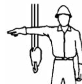
Swing Arm extended, point with finger in direction of swing of boom.
