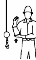
Use Whip Line (Auxiliary Hoist) Tap elbow with open hand; then use regular signals.
