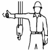
Raise the Boom and Lower the Load With arm extended, thumb pointing up, flex fingers in and out as long as load movement is desired.
