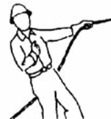
Extend Boom (Telescoping Booms) One hand Signal. One fist in front of chest with thumb tapping chest.
